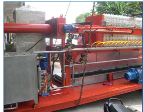
Fully Automatic Membrane Squeezing System Complete With Process Valves, Squeezing Pump, Squeezing Tank
