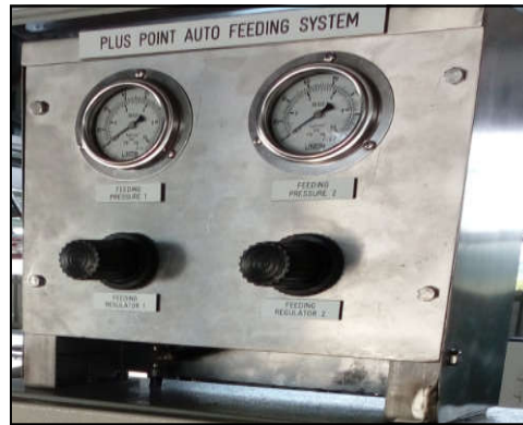
Control Panel With Built In Pneumatic Step Control System For Automatic Feeding By Air Operated Diaphragm Pump.
