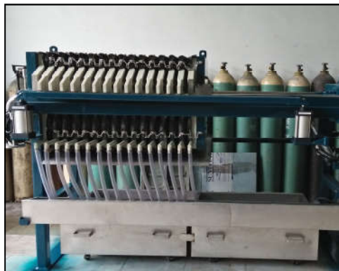
Filter Cake Vibrator Placed Below The Snatch And Latch Plate Shifter System For Dislodging Of Filter Cake
