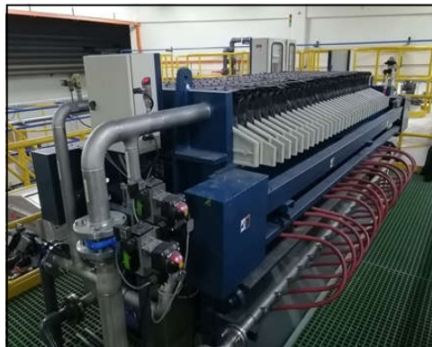
Fully Automatic Feeding and Squeezing System Complete with Process Valves
