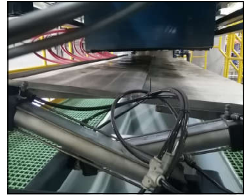
Pneumatically Operated Automatic Drip Tray For Collection Of Filtrate Dripping During Filtration.
