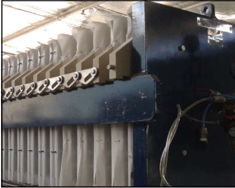
Snatch and Latch Plate Opening System Enables More Efficient Filter Plate Opening And Saves Time
