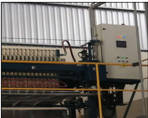
Control Panel With Built IN Touch Screen For More Simple Filter Press Operation
