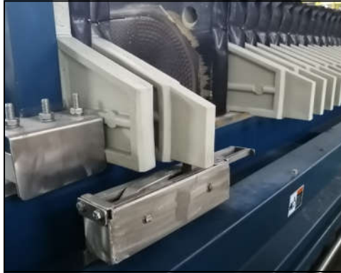
Plate Shifter System for Fully Automatic Operation
