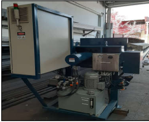
Customized Hydraulic Cylinder And Hydraulic Power Pack With Radial Piston Pump For Lower Closing Pressure And Reliable Operation
