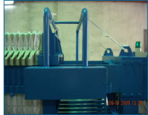
Cost Saving Pneumatically Operated Plate Shifter System For Semi Automatic Operation
