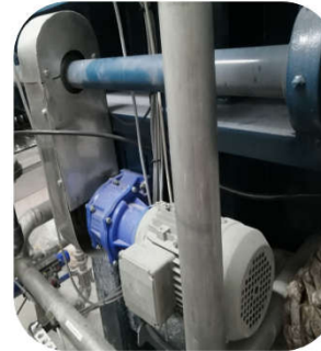
MOTORIZED PLATE SHIFTER FOR CAKE DISCHARGING → Protects Plate Handles
