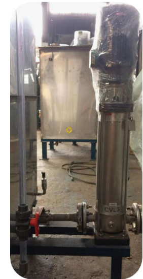
INVERTER CONTROL FOR T-PORT VALVE MEMBRANE FOR SQUEEZING PROCESS → Allow Pressure Regulation for More Uniform Cake
