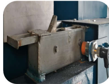
MOTORIZED PLATE SHIFTER FOR CAKE DISCHARGING → Protects Plate Handles
