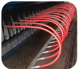
Water Squeezing Piping (Up to 15 bars)
